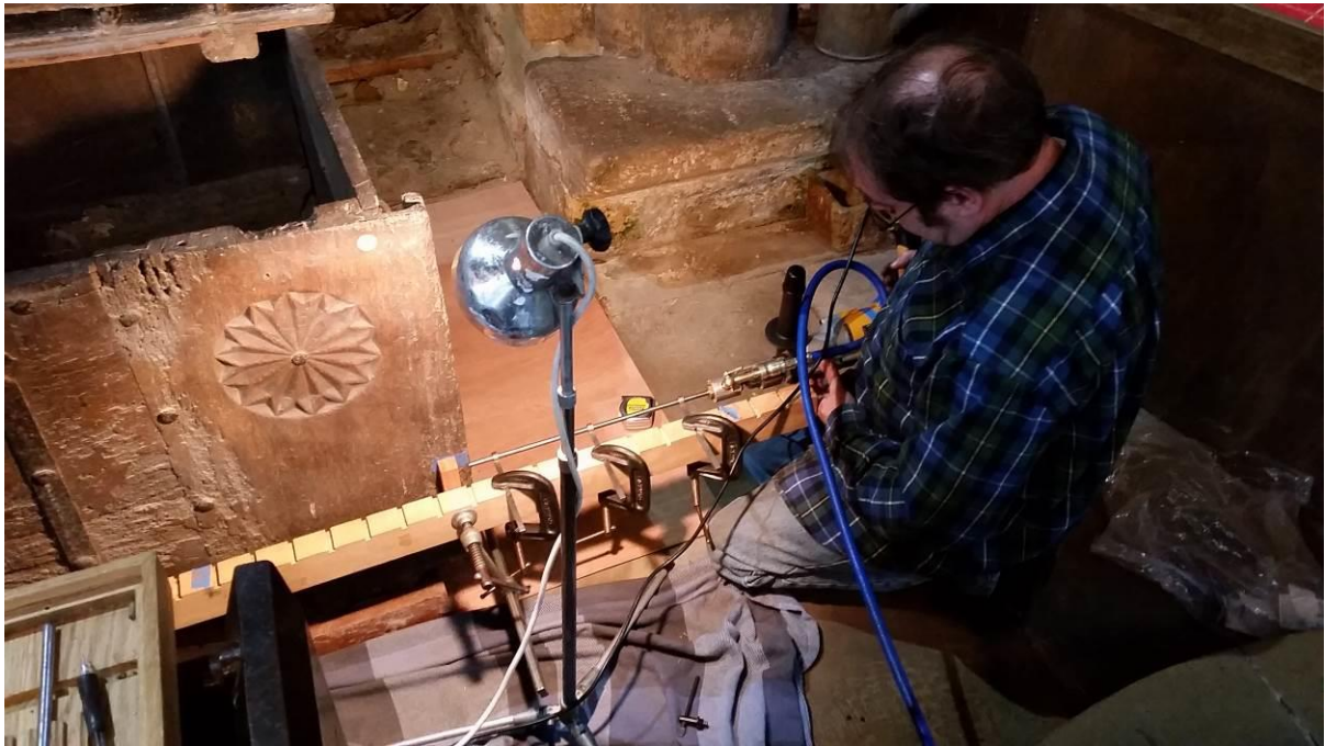
Figure 9: Right front stile of chest ( Inm8 ) being drilled (photo Amy Boyce)
