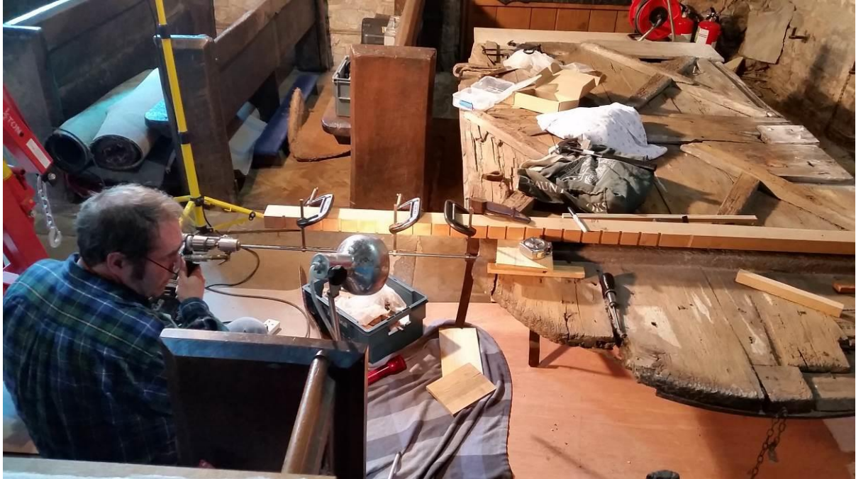
Figure 2: Door being drilled with micro-borer (photo Amy Boyce)
