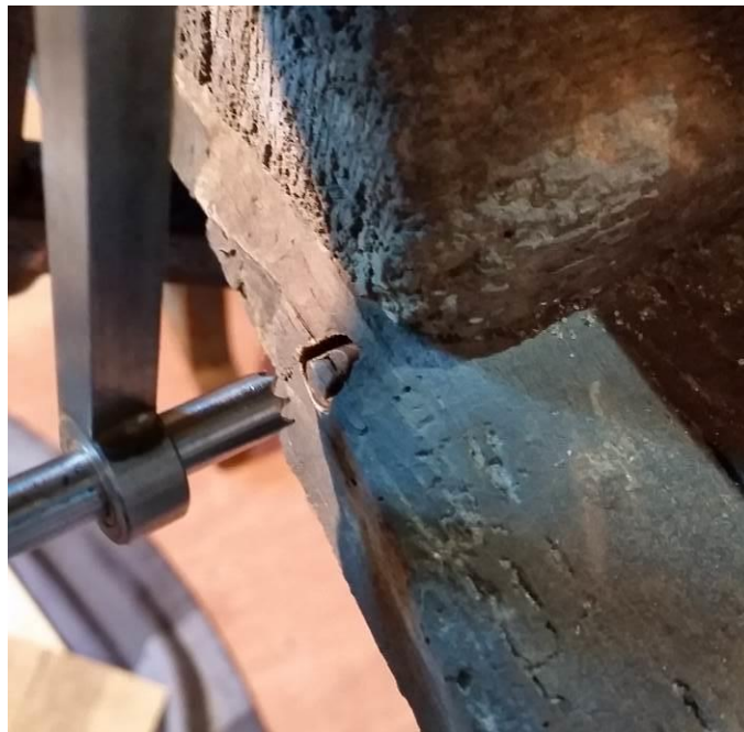
Figure 3: Tip of drill in guide where entering edge of board (photo Amy Boyce)
