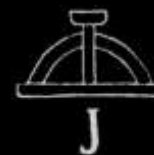
Morton: Pickford type 3.E variant short-headed bellframe formerly in C18th tower. Undated but probably from previous church.
